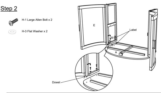
Repeat Step-1 to assembly Right Door (E). Engage all hardware, then loosely tighten using provided Allen Key (T-1). Do not yet fully tighten.
