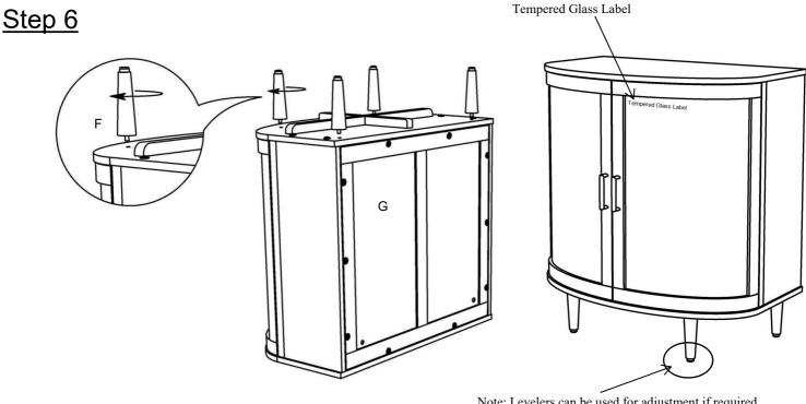
Note: Levelers can be used for adjustment if required
