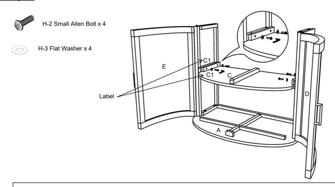
Using a second person for assistance, carefully position the Inner Shelf (C) upside down so that its holes align with pre-drilled holes in both the Left and Right Doors (D and E). Ensure the labels match accordingly (C1 with C1). Secure the connections using Small Allen bolts (H-2) and Flat Washers (H-3), stacking the hardware in order as shown. Engage all hardware, then loosely tighten using provided Allen key (T-1). Do not yet fully tighten.
