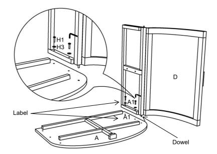
Place the Top Panel (A) upside down onto a padded, non-marring surface. Align the holes in Left Door (D) with the pre-drilled holes in Top Panel (A). Ensure the labels match accordingly (A1 with A1) and that the dowel aligns with its corresponding pre-drilled holes. Secure the connection using Large Allen Bolts (H-1) and Flat Washers (H-3), stacking the hardware in the order as shown. Engage all hardware, then loosely tighten using provided Allen Key (T-1). Do not yet fully tighten.
